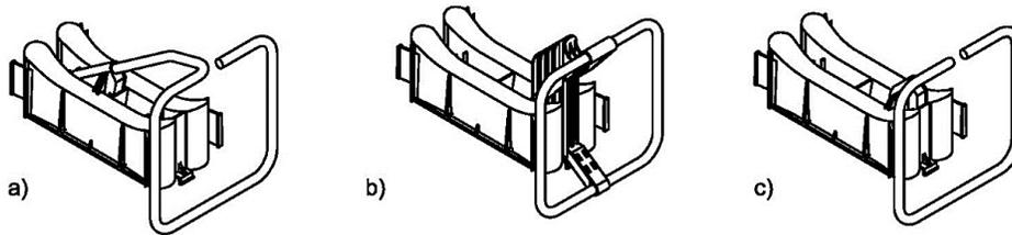
**FIGURE 7—CONCRETE COMPRESSION BEARING (CCB) WITH SPECIAL STIRRUP**
