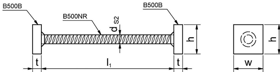
**FIGURE 8—STEEL COMPRESSION BEARING (SCB)**
