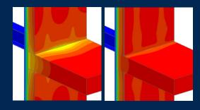
LEFT: Standard uninsulated structural connection. Exterior temperature "seeps through" (yellow).
