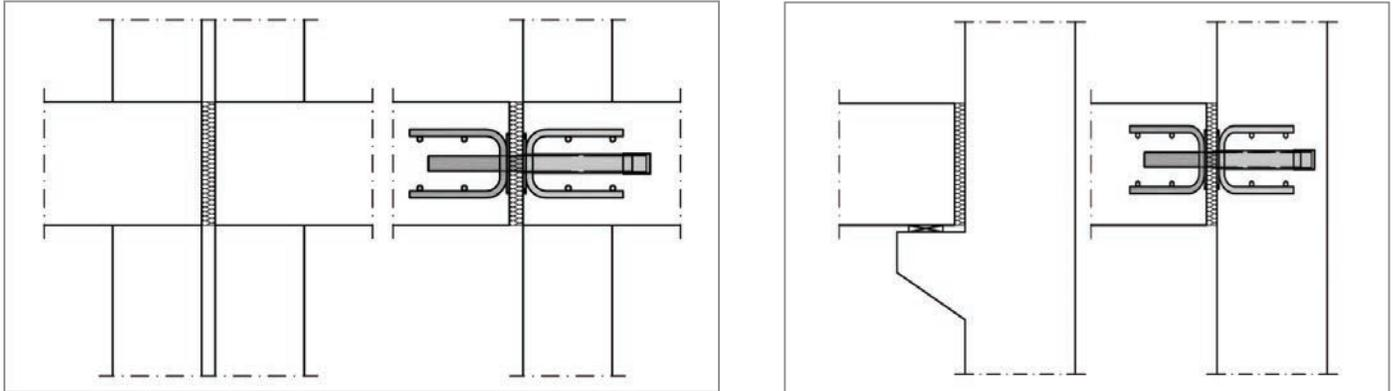
Schöck Dorn Dowels vary in diameter from 16mm to 42mm (5/8" to 1 5/8") with a shear strength of up to 250kN (56.2 kips), depending on the structural element thickness and expansion joint width. Schöck can provide design assistance when required.
