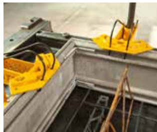
2. Connect corners and fix to the table
