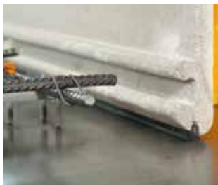
1. Schöck ASE with seal positioned on the form table
