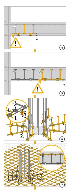
④ The end of the rods must be in one line with the face of the column.
