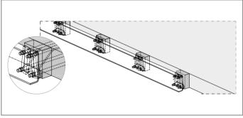
Fig. 18: Principle use of a continuous steel jig
