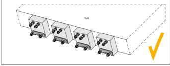
Fig. 22: Schöck Isokorb® type KS: Reliable and correct setting while pouring the concrete ensures the tolerance accuracy is maintained.
