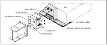
Fig. 23: Usage of a stub bracket to overcome the facade thickness and to allow for horizontal and vertical tolerances
