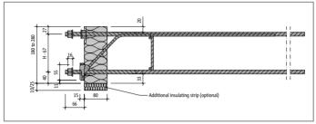
Fig. 9: Schöck Isokorb® type KS14-VV: Product cross section
