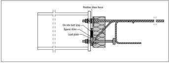
Fig. 30: Schöck Isokorb® type KS: On-site butt stop for transferring shear forces
