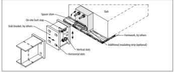
Fig. 12: Usage of a stub bracket to overcome the facade thickness and to allow for horizontal and vertical tolerances
