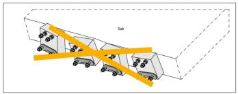
Fig. 21: Schöck Isokorb® type KS: Twisted and displaced elements that were poorly secured while the concrete was being poured
