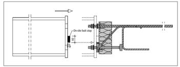
Fig. 29: Schöck Isokorb® type KS: Assembly of steel beam with on-site butt-stop
