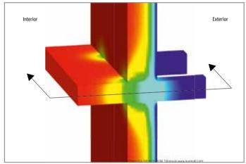
Fig. 1: Illustration of a local thermal bridge on a point balcony connection
