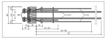
Fig. 6: Schöck Isokorb® type KS14-V8: Plan view
