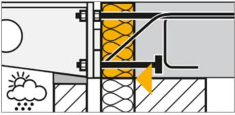
Fig. 13: Positioning of the product in cavity walls
