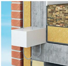
Isokorb® structural thermal breaks for concrete parapet construction are insulated, engineered assemblies with stainless steel rebar for casting into concrete roof slabs.
