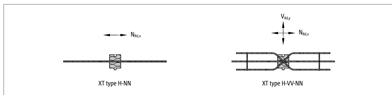
Fig. 217: Schöck Isokorb® XT type H: Type selection
