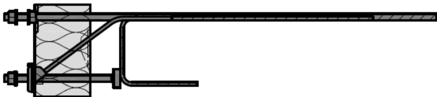
Fig.5: Schöck Isokorb® XT types SK-M1-V1 and SK-M1-V2
