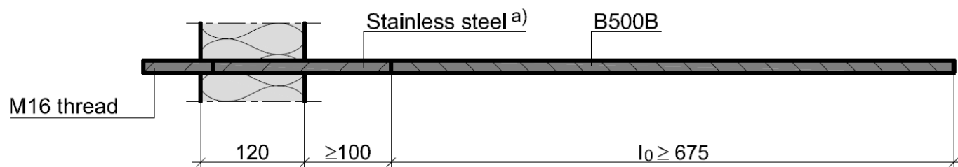
Fig.39: Tensile and compression bars 2 x 2 Ø 14
