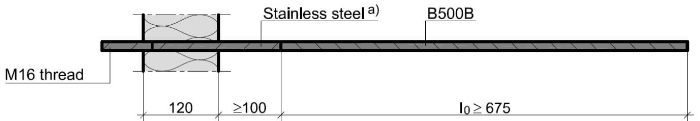
Fig.33: Tensile bars 2 \varnothing 14
