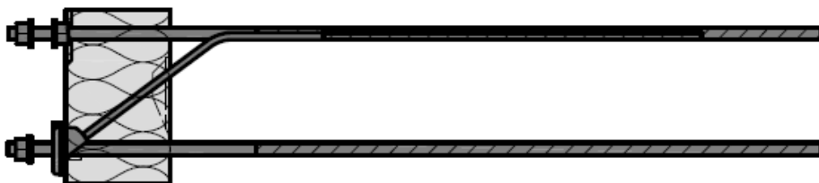
Fig.6: Schöck Isokorb® XT type SK-MM1-VV1
