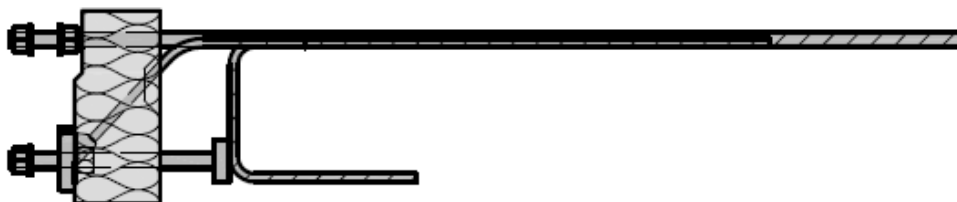
Fig.1: Schöck Isokorb® T types SK-M1-V1 and SK-M1-V2
