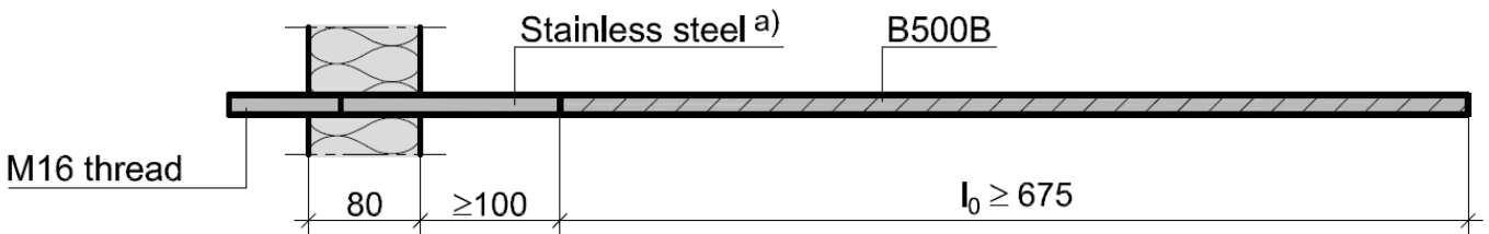
Fig.11: Tensile bars 2 \varnothing 14
