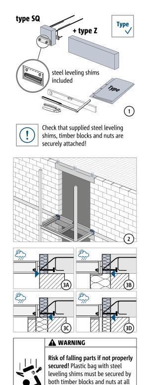
times. Steel leveling shims for use
