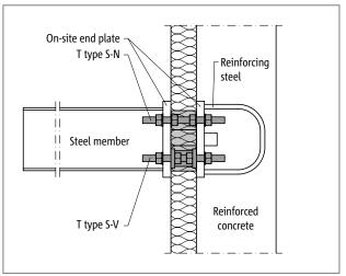
Fig. 102: Schöck Isokorb® T type S-N and T type S-V: for connection of steel structures to reinforced concrete
