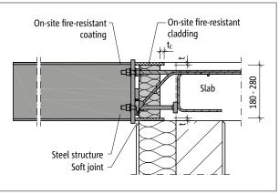
Fig. 37: Schöck Isokorb® T type SK: on site fire-resistant cladding of the connection when using steel structures with fire-resistant coating; cross-section
