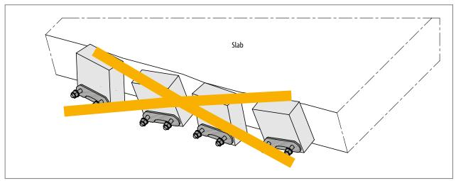
Fig. 75: Schöck Isokorb® T type SQ: Twisted and displaced elements that were poorly secured while the concrete was being poured
