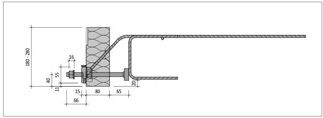
Fig. 84: Schöck Isokorb® T type SQ-V1: Cross section of the product
