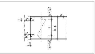
Fig. 130: Flush end plate T type S: Geometric input values from calculation; view
