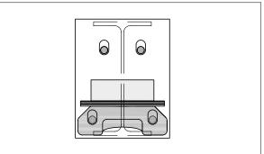
Fig. 28: Schöck Isokorb $^{\otimes}$  T type SK: Adding design shims on the load plate will raise the steel beam by up to 20 mm
