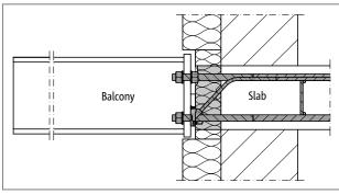
Fig. 9: Schöck Isokorb® T type SK: Connection to the reinforced concrete floor; insulating element within the outer insulation
