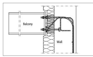
Fig. 12: Schöck Isokorb® T type SK-WU-M1: Special construction for wall connection on the basis of the shear force bearing levels M1 for wall thicknesses from 200 mm
