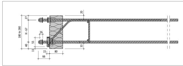
Fig. 35: Schöck Isokorb® T type SK-MM1-VV1: Cross section of the product
