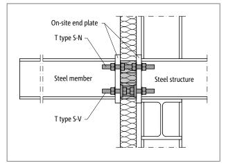
Fig. 98: Schöck Isokorb® T type S-N and T type S-V:for cantilevered steel structures
