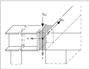
Fig. 68: Schöck Isokorb® T type SQ: Direction of internal forces and moments
