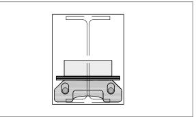
Fig. 78: Schöck Isokorb® T type SQ: Shims on the load plate raise the position of the steel beam by up to 20 mm
