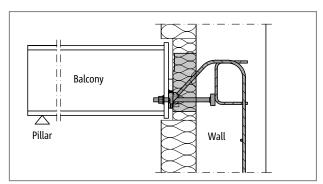
Fig. 65: Schöck Isokorb® T Type SQ-WU: Special design; required for the connection to a reinforced concrete wall
