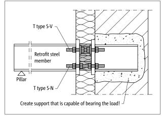
Fig. 103: Schöck Isokorb® T type S-N and T type S-V: for retrofitteds supported steel structure; for further renovation examples see p. 96
