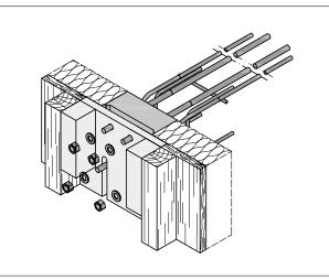
Fig. 29: Schöck Isokorb® type KS: Representation with installation aid
