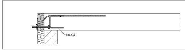
Fig. 88: Schöck Isokorb® T type SQ: On-site reinforcement: Cross section
