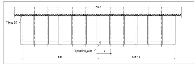
Fig. 18: Schöck Isokorb® T type SK: Maximum expansion joint spacing e
