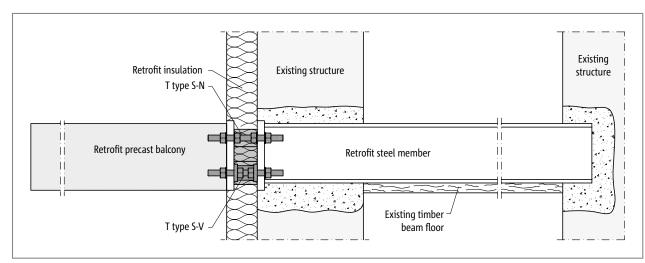
Fig. 135: Schöck Isokorb® T type S-N and T type S-V: Retrofitted cantilevered precast balcony; connected to retrofitted steel beam; internal screw connection
