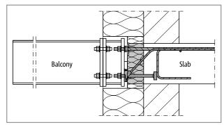
Fig. 14: Schöck Isokorb® T type SK: Connection of the steel member to an adapter that equalises the thickness of the outer insulation
