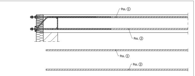
Fig. 40: Schöck Isokorb® T type SK-MM1: On-site reinforcement: Cross section
