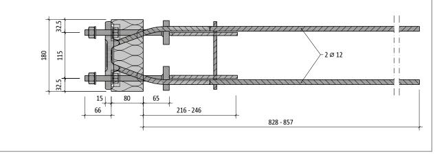
Fig. 83: Schöck Isokorb® T type SQ-V3: Plan view
