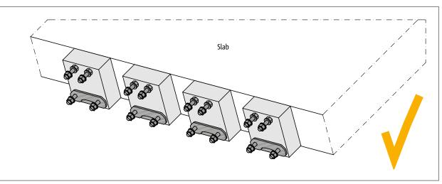
Fig. 26: Schöck Isokorb® T type SK: Reliable and correct setting while pouring the concrete ensures the tolerance accuracy is maintained.
