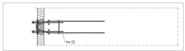
Fig. 89: Schöck Isokorb® T type SQ: On-site reinforcement: Plan view
