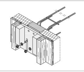
Fig. 79: Schöck Isokorb® T type SQ: Representation with installation aid
