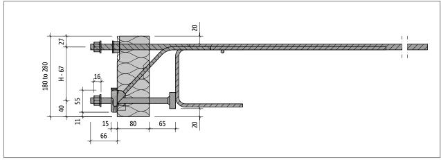
Fig. 34: Schöck Isokorb® T type SK-M1-V1: Cross section of the product
