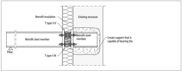
Fig. 137: Schöck Isokorb® T type S-N and T type S-V: Retrofitted supported steel balcony; connected to retrofitted wall support
