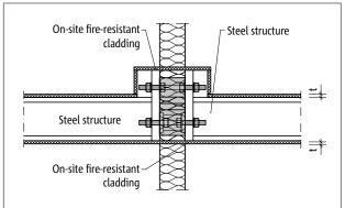
Fig. 6: Fire protection Schöck Isokorb $^{\circ}$  T type S: On-site fire protection cladding for overlaying face plates; section
