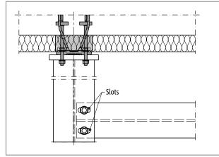
Fig. 71: Schöck Isokorb® T type SQ: Expansion joint detail to ensure movement during temperature expansion
