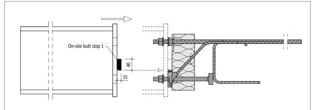
Fig. 55: Schöck Isokorb® T type SK: Mounting the steel member
