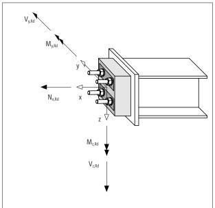
Fig. 108: Schöck Isokorb® T type S: Sign convention for design
