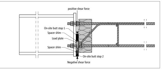
Fig. 58: Schöck Isokorb® T type SK: On-site dogs for the transfer of the shear force
