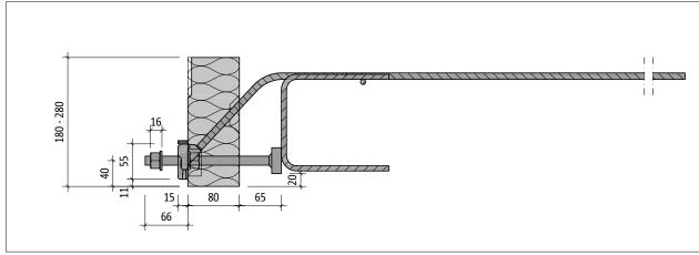
Fig. 85: Schöck Isokorb® T type SQ-V2: Cross section of the product
