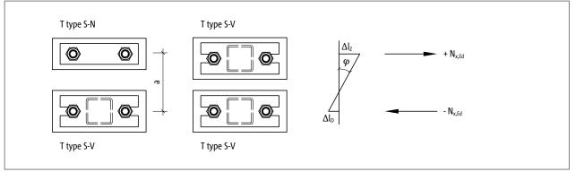
Fig. 109: Schöck Isokorb<sup>®</sup> T type S-N + T type S-V and 2 × T type S-V: Torsion angle  $\varphi \approx \tan \varphi = (\Delta l_2 + \Delta l_2) / a$
