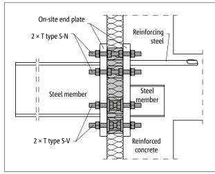
Fig. 101: Schöck Isokorb® T type S-N and T type S-V: for connection of steel structures to reinforced concrete
