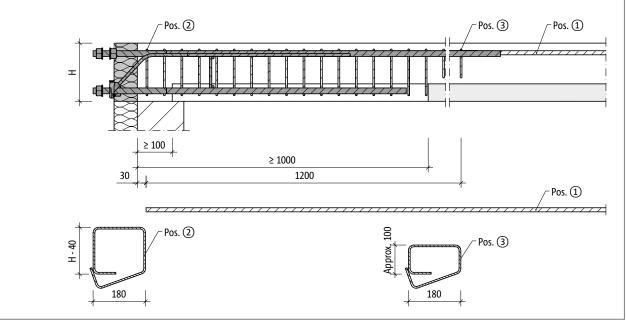
Fig. 47: Schöck Isokorb® T type SK-MM2: On-site reinforcement with stirrup Ø 6 mm for semi-precast construction; cross-section
