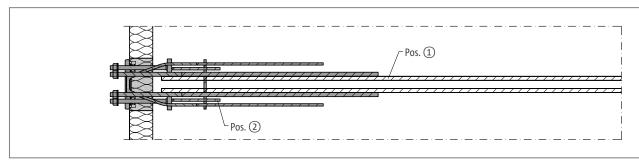
Fig. 39: Schöck Isokorb® T type SK-M1: On-site reinforcement: Plan view
