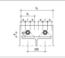
Fig. 128: Protruding end plate T type S: geometric input values from calculation; view
