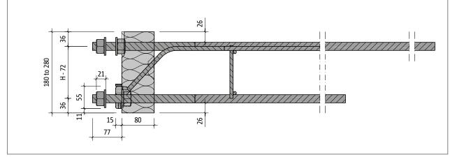
Fig. 36: Schöck Isokorb® T type SK-MM2-VV1: Cross section of the product
