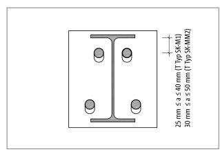
Fig. 54: Schöck Isokorb® T type SK-MM2...-H200: End plate connection to IPE220 beam.
