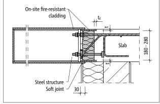
Fig. 1: Schöck Isokorb® T type SK: on site fire-resistant cladding T type SK and steel structure; cross section
