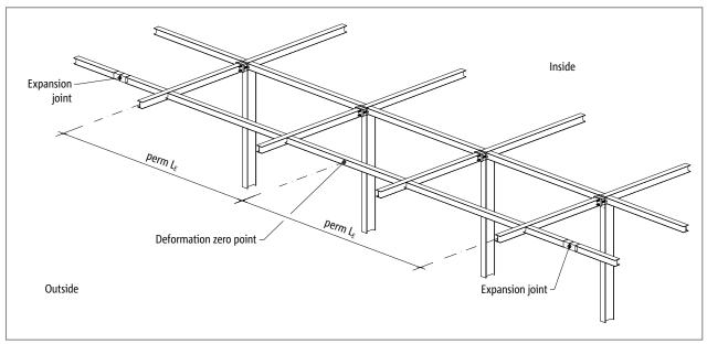
Fig. 110: Schöck Isokorb® T type S: Load influence length of the outer construction subjected to temperature expansion
