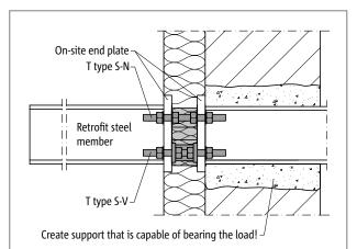
Fig. 104: Schöck Isokorb® T type S-N and T type S-V:for retrofitteds cantilevered steel structure; for further renovations examples see p. 96
