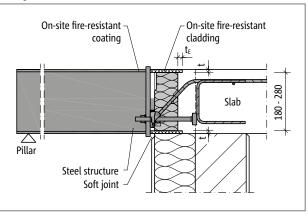
Fig. 87: Schöck Isokorb® T type SQ: on site fire-resistant cladding of the connection when using steel structures with fire-resistant coating; cross-section
