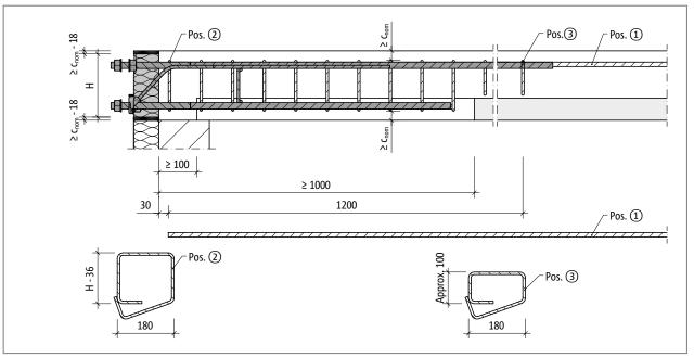
Fig. 48: Schöck Isokorb® T type SK-MM2: On-site reinforcement with stirrup Ø 8 mm for semi-precast construction; cross section
