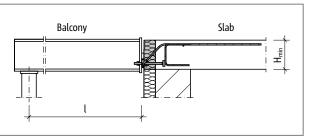
Fig. 69: Schöck Isokorb® T type SQ: Static system
