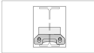
Fig. 77: Schöck Isokorb® T type SQ: on-site shim lies directly on the load plate
