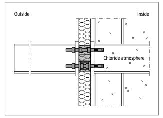
Fig. 105: Schöck Isokorb® T type S with cap nuts: for cantilevered steel structures, chloride atmosphere inside
