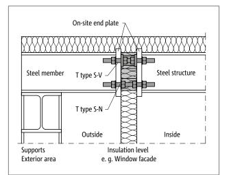
Fig. 97: Schöck Isokorb® T type S-N and T type S-V:for separation within the structural system
