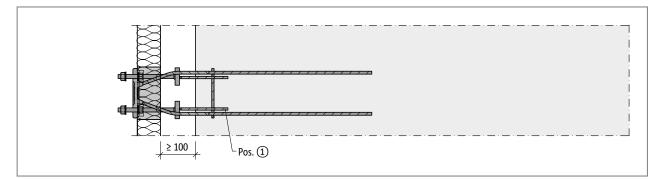
Fig. 91: Schöck Isokorb® T type SQ: On-site reinforcement for semi-precast construction: Plan view
