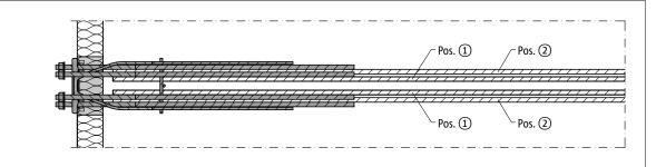
Fig. 41: Schöck Isokorb® T type SK-MM1: On-site reinforcement: Plan view
