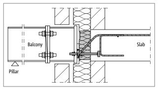
Fig. 62: Schöck Isokorb<sup>®</sup> T type SQ: insulating element within the core insulation zone; steel stub adjuster between the Isokorb<sup>®</sup> and the balconyfor flexible construction workflow
