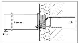
Fig. 66: sokorb® T type SQ:Using the ceiling floorion, the insulation body is flush with the insulation of the wall on the outside.outside, the lateral edge distances must be taken into account.
