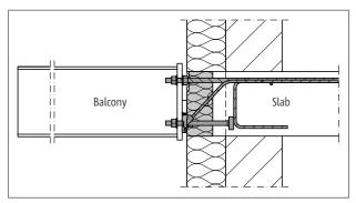
Fig. 13: Schöck Isokorb<sup>®</sup> T type SK: With the aid of the floor extension, the insulating element ends flush with the wall insulation; the spacing at the edges must be taken into consideration.
