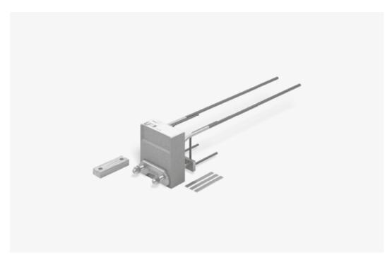
Schöck Isokorb® T type SQ Suitable for supported steel balconies and canopies. It transfers positive shear forces.
