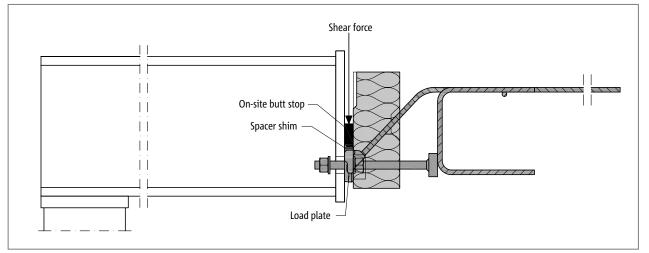
Fig. 94: Schöck Isokorb® T type SQ: On-site butt stop for transferring shear forces
