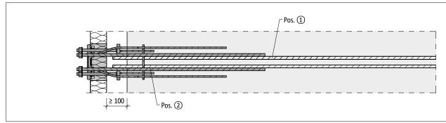
Fig. 46: Schöck Isokorb® T type SK-M1: On-site reinforcement for semi-precast construction: Plan view
