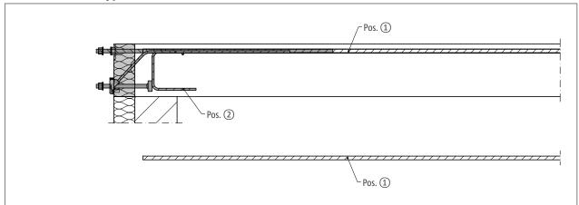
Fig. 38: Schöck Isokorb® T type SK-M1: On-site reinforcement: Cross section
