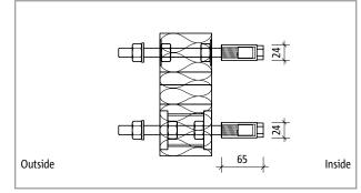
Fig. 140: Schöck Isokorb® T type S with cap nuts: Isometry; internal atmosphere containing chloride
