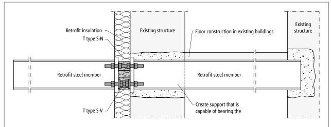
Fig. 132: Schöck Isokorb® T type S-N and T type S-V: Retrofitted cantilevered steel balcony; connected to retrofitted steel beam
