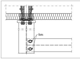
Fig. 19: Schöck Isokorb® T type SK: Expansion joint detail to ensure movement during temperature expansion
