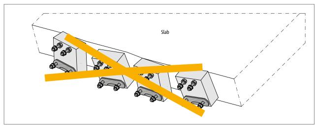
Fig. 25: Schöck Isokorb® T type SK: Twisted and displaced elements that were poorly secured while the concrete was being poured
