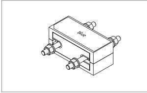
Fig. 121: Schöck Isokorb® T type S-V-D16: Isometry; colour code T type S-V: Blue
