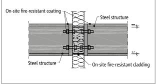
Fig. 7: Fire protection Schöck Isokorb® T type S: On-site fire protection cladding T type S, fire protection coated steel structure; section
