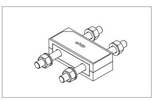
Fig. 116: Schöck Isokorb® T type S-N-D22: Isometry; colour code T type S-N: White
