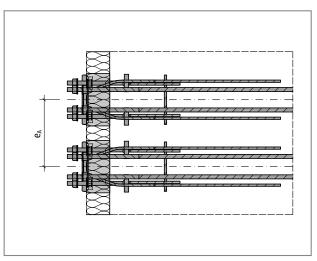
Fig. 22: Schöck Isokorb® T type SK: Centre-to-centre distance
