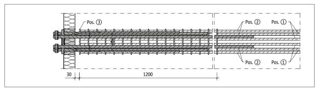
Fig. 44: Schöck Isokorb® T type SK-MM2: On-site reinforcement: Plan view
