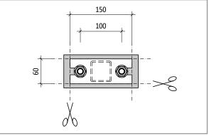
Fig. 123: Schöck Isokorb $^{\otimes}$ T type S-N: Dimensions after trimming the insulation body
