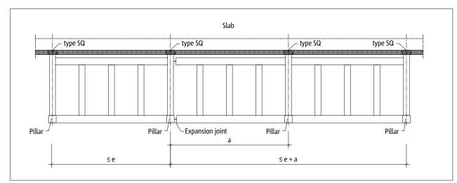
Fig. 70: Schöck Isokorb® T type SQ: Maximum expansion joint spacing e and lateral overhang a
