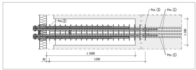
Fig. 49: Schöck Isokorb® T type SK-MM2: On-site reinforcement for semi-precast construction, plan view
