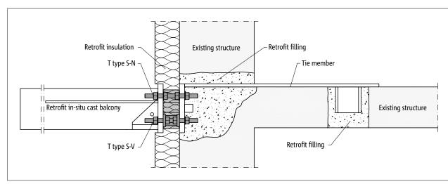
Fig. 136: Schöck Isokorb<sup>®</sup> T type S-N and T type S-V: Retrofitted cantilevered in situ concrete balcony; connected to existing reinforced concrete ceiling with tie member
