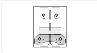
Fig. 27: Schöck Isokorb® T type SK: On-site butt stop lies directly on the load plate
