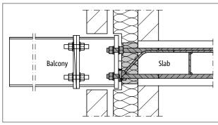
Fig. 10: Schöck Isokorb® T type SK: Insulating element within the core insulation; on-site adapter between the Isokorb® and the balconyto enable flexible installation
