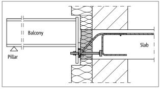
Fig. 64: Isokorb® T type SQ:Barrier-free access due to height offsetoffset
