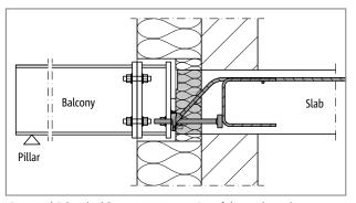
Fig. 67: Schöck Isokorb\* T type SQ: Connection of the steel member to an adapter that equalises the thickness of the outer insulation
