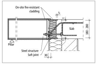
Fig. 3: Schöck Isokorb® T type SQ: on site fire-resistant cladding T type SQ and steel structure; cross-section
