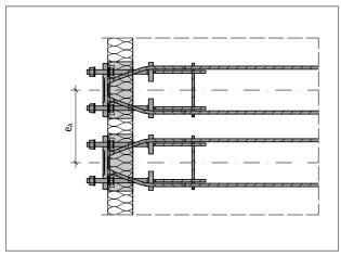
Fig. 74: Schöck Isokorb® T type SQ: Centre-to-centre distance
