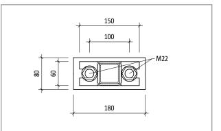
Fig. 120: Schöck Isokorb® T type S-V-D22: Product elevation
