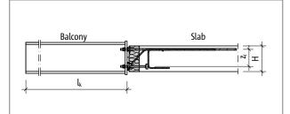
Fig. 16: Schöck Isokorb<sup>®</sup> T type SK: Structural system; Design values refer to the presented cantilever length  $l_k$
