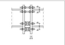
Fig. 127: End plate T type S: Geometric input values from table; cross-section
