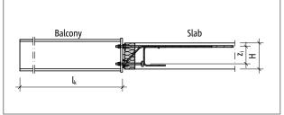
Fig. 60: Schöck Isokorb® T type SK: Structural system; Design values refer to the presented cantilever length  $l_{\rm k}$
