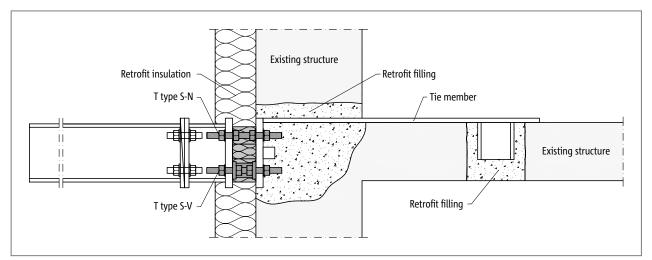
Fig. 133: Schöck Isokorb<sup>®</sup> T type S-N and T type S-V: Retrofitted cantilevered steel balcony with adapter; connected to existing reinforced concrete floor with tie member
