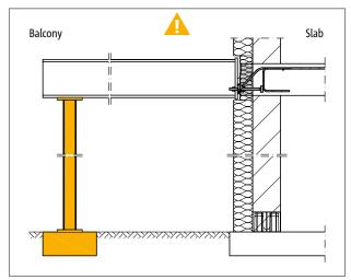
Fig. 95: Schöck Isokorb® T type SQ: Continuous support needed
