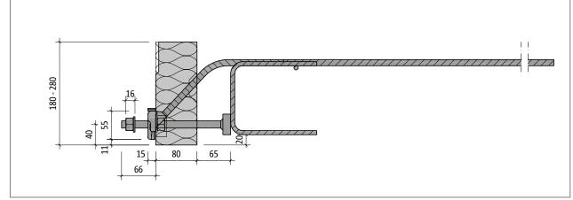
Fig. 86: Schöck Isokorb® T type SQ-V3: Cross section of the product
