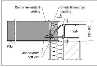
Fig. 4: Schöck Isokorb® T type SQ: on site fire-resistant cladding of the connection when using steel structures with fire-resistant coating; cross-section
