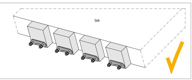
Fig. 76: Schöck Isokorb® T type SQ: Reliable and correct setting while pouring the concrete ensures the tolerance accuracy is maintained.
