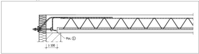
Fig. 90: Schöck Isokorb® T type SQ: On-site reinforcement for semi-precast construction: Cross section
