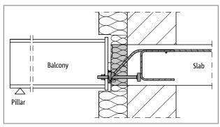
Fig. 63: Schöck Isokorb<sup>®</sup> T type SQ: Connection to reinforced concrete inner slab; insulating element within the core insulation zone.
