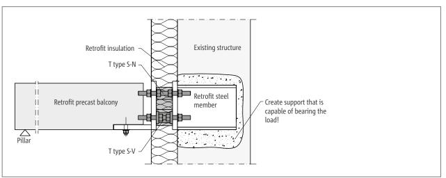
Fig. 138: Schöck Isokorb® T type S-N and T type S-V: Retrofitted supported precast balcony; connected to retrofitted steel beam
