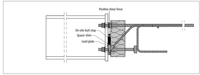
Fig. 56: Schöck Isokorb® T type SK: On-site butt stop for transferring shear forces
