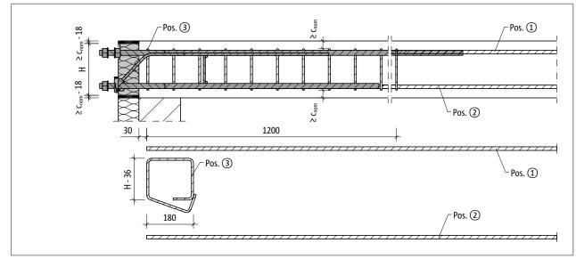
Fig. 43: Schöck Isokorb® T type SK-MM2: On-site reinforcement with stirrup Ø 8 mm; section
