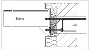
Fig. 11: Isokorb® T type SK:Barrier-free access due to height offsetoffset
