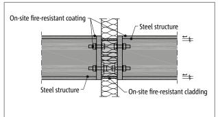
Fig. 125: Fire protection Schöck Isokorb® T type S: On-site fire protection cladding T type S, fire protection coated steel structure; section
