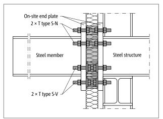
Fig. 99: Schöck Isokorb® T type S-N and T type S-V:for cantilevered steel structures
