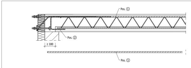
Fig. 45: Schöck Isokorb® T type SK-M1: On-site reinforcement for semi-precast construction: Cross section
