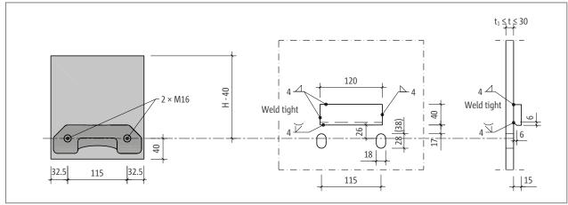
Fig. 92: Schöck Isokorb® T type SQ: Design of the fixing plate connection
