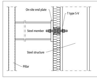
Fig. 96: Schöck Isokorb® T type S-V:for supported steel structures
