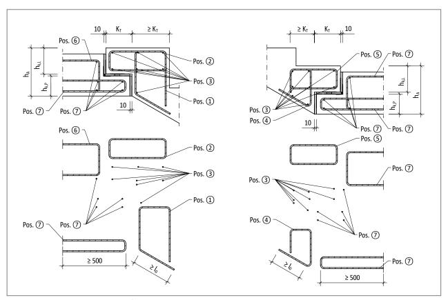
Fig. 77: Schöck Tronsole  $^{\circ}$  type F: On-site reinforcement with superelevated connection
