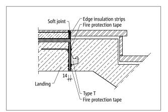
Fig. 14: Schöck Tronsole® Type T: Fire-protection version
