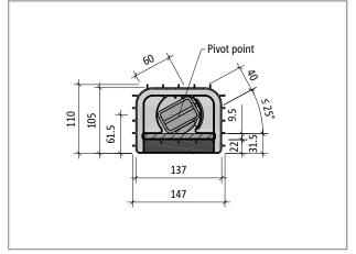
Fig. 105: Schöck Tronsole  $^{\circ}$  type Q: Product cross-section with rotated load-bearing element
