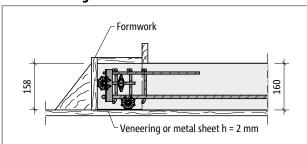
Fig. 151: Schöck Tronsole® type Z: Production of a support corbelt on the fully precast landing; landing slab thickness h = 160 mm
