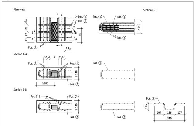
Fig. 108: Schöck Tronsole® type Q: On-site reinforcement
