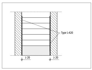
Fig. 194: Schöck Tronsole® type L-420: Taking into account installation toler-
