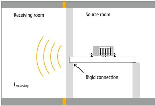
Fig. 10: Determination of the standard landing impact sound pressure level  $L_{n0,landing}$  of the reference landing without the impact sound insulation ele-
