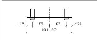
Fig. 35: Schöck Tronsole  $^{\circ}$  type T-V2-H...-L1001 to L1300: Product layout
