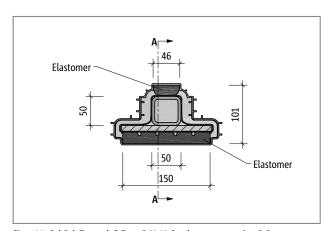
Fig. 132: Schöck Tronsole® Type P-V+V: Product cross-section B-B
