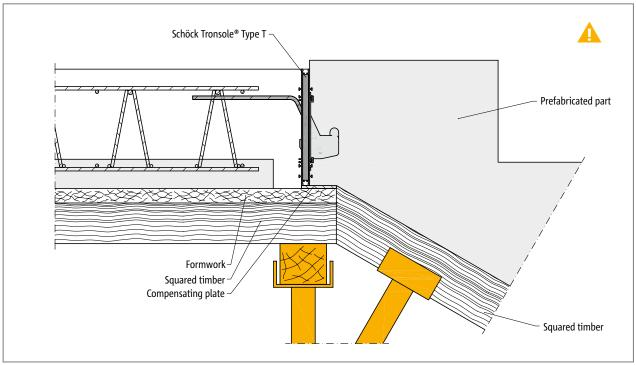
Fig. 58: Schöck Tronsole® Type T: Supports coloured yellow
