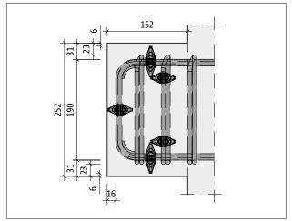
Fig. 163: Schöck Tronsole® type Z: Plan view of a concrete landing with integrated load-bearingelement
