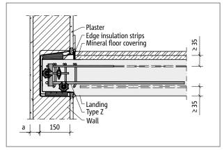
Fig. 19: Schöck Tronsole® type Z: Fire protection configuration
