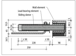
Fig. 104: Schöck Tronsole® type Q: Product section A-A
