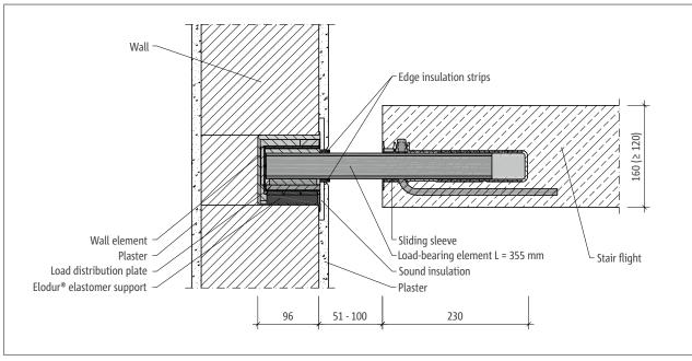
Fig. 95: Schöck Tronsole® type Q-FV-XL or Q-A2-XL: Installation cross-section
