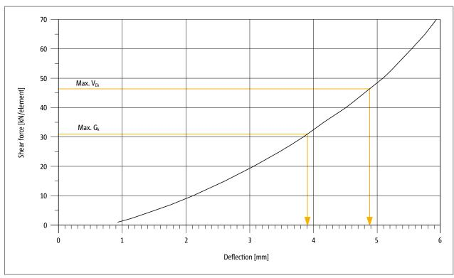
Fig. 138: Schöck Tronsole $^{\circ}$  Type P: Deformation of the Elodur $^{\circ}$  elastomeric bearing with a positive  $V_{\text{Ek,z}}$
