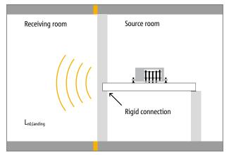
Fig. 4: Determination of the standard landing impact sound pressure level  $L_{n0,landing}$  of the reference landing without the impact sound insulation element
