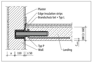
Fig. 18: Schöck Tronsole® Type P: Fire-protection version
