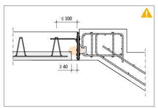
Fig. 54: Schöck Tronsole® type T: Installation in combination with prefabricated floors, compression joint on floor side
