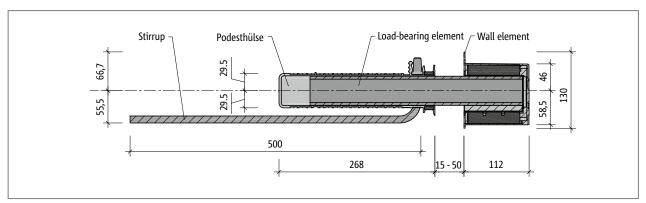
Fig. 131: Schöck Tronsole® Type P: Product section A-A
