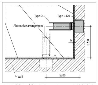
Fig. 99: Schöck Tronsole® type Q: Component arrangement, Detail A, joint width b=15 mm with in-situ concrete, with precast stair flights the necessity of an additional installation tolerance is to be checked by the planner
