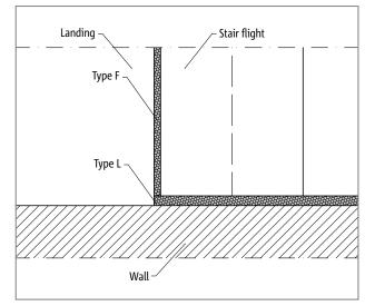
Fig. 68: Schöck Tronsole® type F: Element configuration, Detail B
