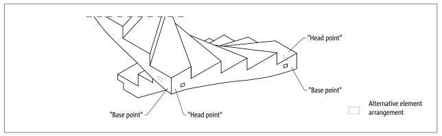
Fig. 109: Schöck Tronsole® type Q: Attachment point in "head point" and "base point"
