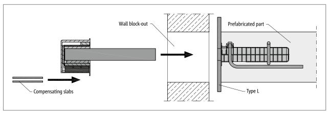
Fig. 114: Schöck Tronsole® type Q: Wall recess with prefabricated construction
