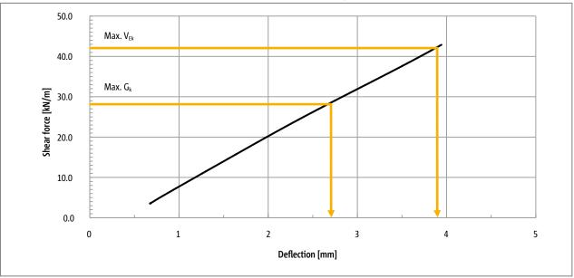
Fig. 185: Schöck Tronsole® type B-V2: Deformation of the Elodur® elastomer support
