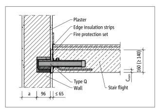
Fig. 17: Schöck Tronsole® type Q: Fire protection configuration
