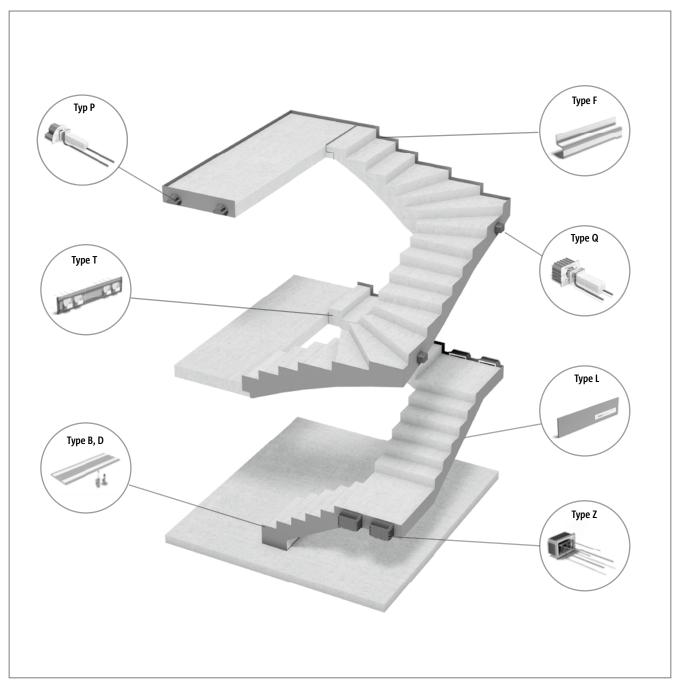
Fig. 1: Sound-insulation system made using Schöck Tronsole®
