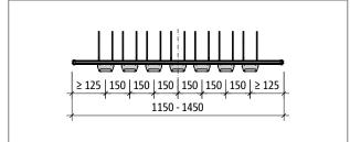
Fig. 43: Schöck Tronsole® type T-V7-H...-L1150 to L1450: Product layout
