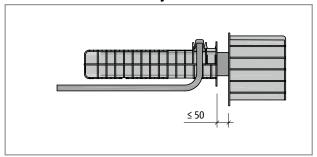
Fig. 90: Schöck Tronsole® type Q: Installation variant joint width ≤ 50 mm
