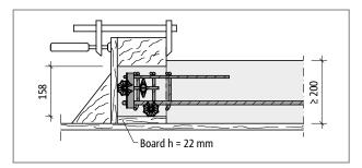
Fig. 153: Schöck Tronsole® Type Z: Constructing a support bracket on a fully precast landing; slab thickness  $h \ge 200 \text{ mm}$
