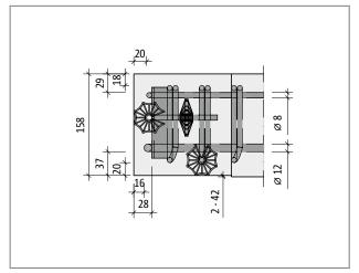
Fig. 162: Schöck Tronsole $^{\otimes}$  type Z: Side view of a concrete landing with integrated load-bearing element
