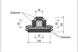
Fig. 133: Schöck Tronsole® Type P-VH+VH: Product cross-section B-B
