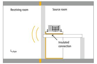
Fig. 7: Determination of the standard flight impact sound pressure level  $L_{\rm n...}$  flight of the reference stair flight with the impact sound insulation element to be checked
