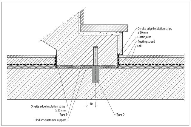
Fig. 172: Schöck Tronsole $^{\otimes}$  type B + type D: Alternative installation
