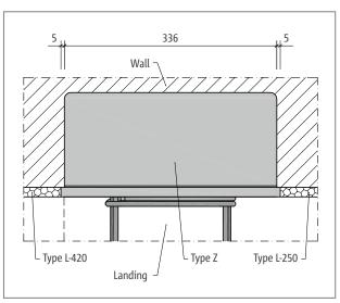
Fig. 159: Schöck Tronsole® type Z: Element configuration, Detail A
