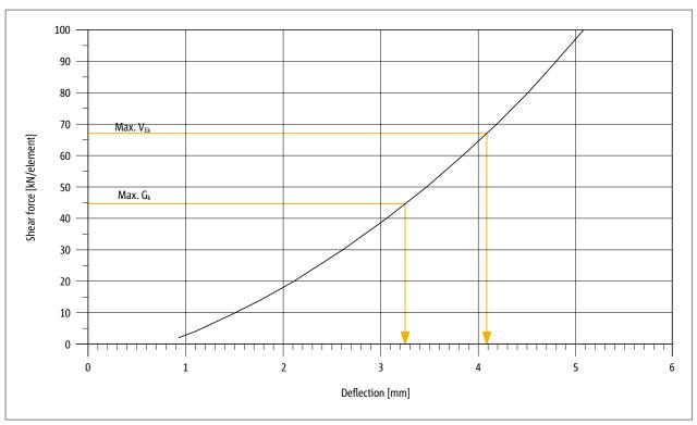
Fig. 140: Schöck Tronsole  $^{\circ}$  Type P: Deformation of the Elodur  $^{\circ}$  elastomeric bearing under a vertical load  $V_{\text{Ek,z}}$  when arranged in pairs
