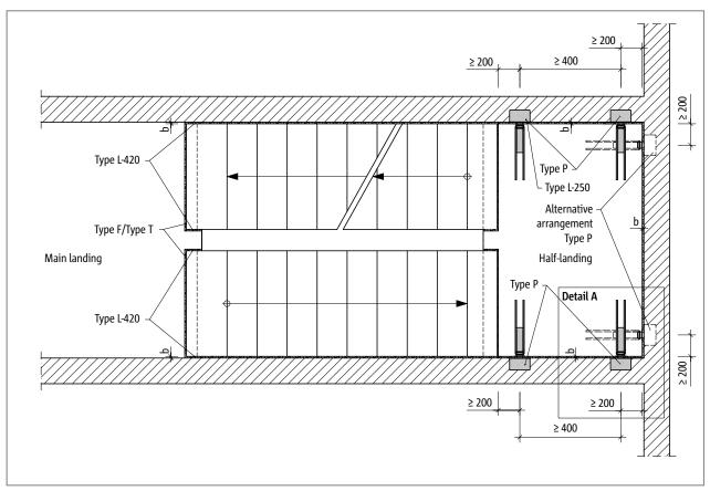
Fig. 124: Schöck Tronsole® Type P: Element arrangement in plan view using Tronsole® Type L
