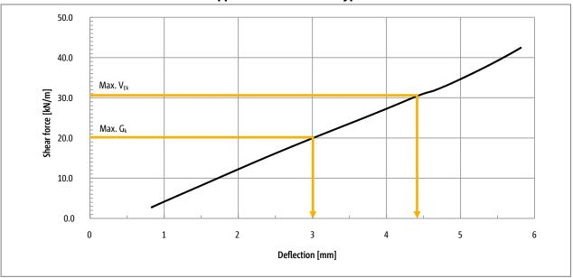
Fig. 81: Schöck Tronsole® type F-V1: Deformation of the Elodur® elastomer support
