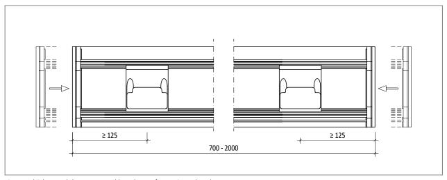
Fig. 61: Schöck Tronsole  $^{\circ}$  type T: Assemble end caps after cutting to length
