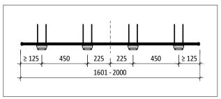
Fig. 39: Schöck Tronsole® type T-V4-H...-L1601 to L2000: Product layout
