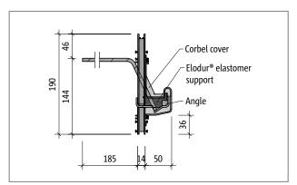
Fig. 33: Schöck Tronsole  $^{\circ}$  type T: Product section T...-H190 through the support bracket
