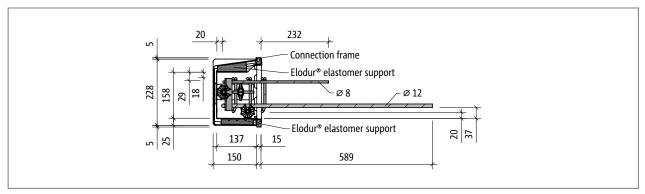
Fig. 161: Schöck Tronsole® type Z-V+V-T respectively type Z-VH+VH-T: Vertical cross-section
