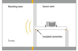
Fig. 9: Determination of the standard landing impact sound pressure level  $L_{n,landing}$  of the reference landing with the impact sound insulation element to be checked
