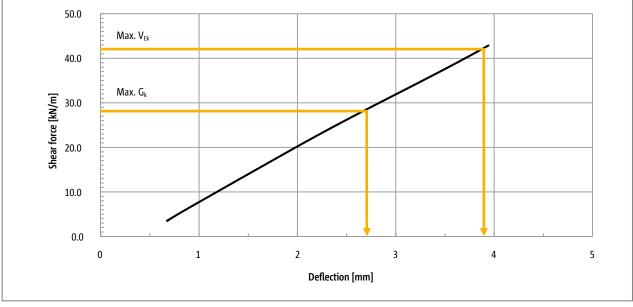
Fig. 82: Schöck Tronsole® type F-V2: Deformation of the Elodur® elastomer support
