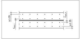
Fig. 84: Schöck Tronsole® type F: Vertical section transverse to the stairs in the area of the corbel support; depiction of the concrete cover c<sub>nom,l</sub>, c<sub>nom,P</sub> and the minimum centre-to-centre distance u of the reinforcement
