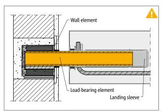
Fig. 142: Schöck Tronsole® Type P: Multi-part product (wall element, load-bearing element, landing sleeve); load-bearing element (yellow) must be installed on the building site.
