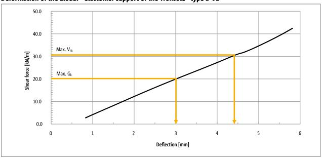
Fig. 184: Schöck Tronsole® type B-V1: Deformation of the Elodur® elastomer support
