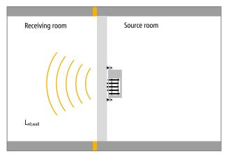
Fig. 8: Determination of the standard wall impact sound pressure level  $L_{n0,wall}$  the reference wall on a test bench
