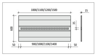
Fig. 178: Schöck Tronsole® type B-V2-L...-B600: Product layout
