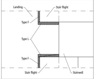
Fig. 67: Schöck Tronsole® type F: Element configuration, Detail A
