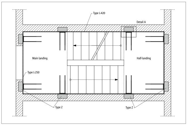
Fig. 158: Schöck Tronsole  $^{\circ}$  type Z: Alternative element configuration in plan view
