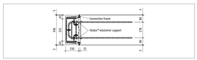
Fig. 160: Schöck Tronsole® type Z-VH+VH-T: Horizontal cross-section
