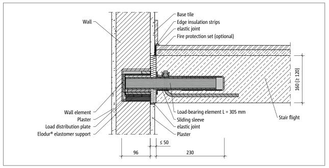
Fig. 94: Schöck Tronsole® type Q-FV or Q-A2: Installation cross-section wall thickness 11.5 cm
