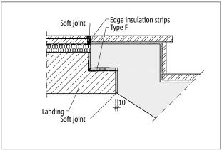
Fig. 15: Schöck Tronsole® Type F: Fire-protection version
