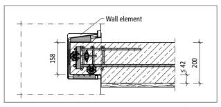
Fig. 149: Schöck Tronsole® type Z: Wall element as stay-in-place formwork; underside of the landing lower than the connection frame of the wall element
