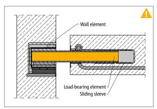
Fig. 112: Schöck Tronsole® type Q: Multi-part product (wall component, load-bearing component, sliding sleeve); load-bearing element (yellow) must be installed on the building site.
