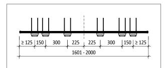
Fig. 42: Schöck Tronsole® type T-V6-H...-L1601 to L2000: Product layout
