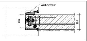
Fig. 148: Schöck Tronsole® type Z: Wall element as stay-in-place formwork; underside of the landing flush with the connection frame of the wall element
