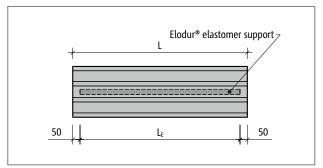
Fig. 182: Schöck Tronsole® type B Representation of lengths L and L<sub>6</sub>; the length of the Elodur® elastomer support is always 10 cm shorter than the length of the Tronsole®.
