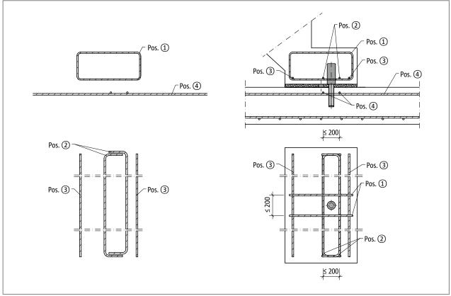
Fig. 183: Schöck Tronsole® type D: On-site reinforcement
