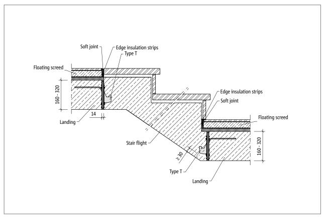
Fig. 24: Schöck Tronsole® type T: Installation cross-section
