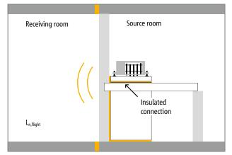
Fig. 11: Determination of the standard flight impact sound pressure level  $L_{n,\cdot}$  flight of the reference stair flight with the impact sound insulation element to be checked
