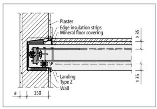
Fig. 168: Schöck Tronsole® type Z: Fire protection configuration
