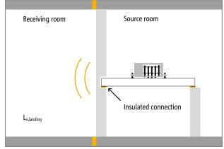
Fig. 5: Determination of the standard landing impact sound pressure level  $L_{n,landing}$  of the reference landing with the impact sound insulation element to be checked
