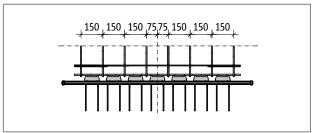
Fig. 50: Schöck Tronsole® type T: Displaced laying pattern of the reinforcement with uneven number of support corbels on the Tronsole®
