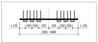
Fig. 41: Schöck Tronsole® type T-V6-H...-L1301 to L1600: Product layout
