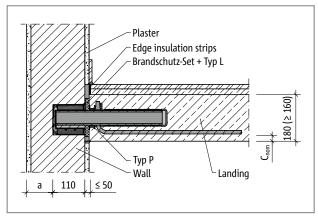
Fig. 144: Schöck Tronsole® Type P: Fire-protection version
