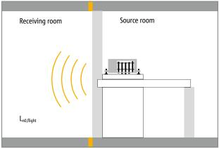
Fig. 6: Determination of the standard flight impact sound pressure level  $L_{n0,-}$  flight of the reference stair flight without the impact sound insulation element
