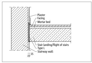
Fig. 20: Schöck Tronsole® Type L: Fire-protection version
