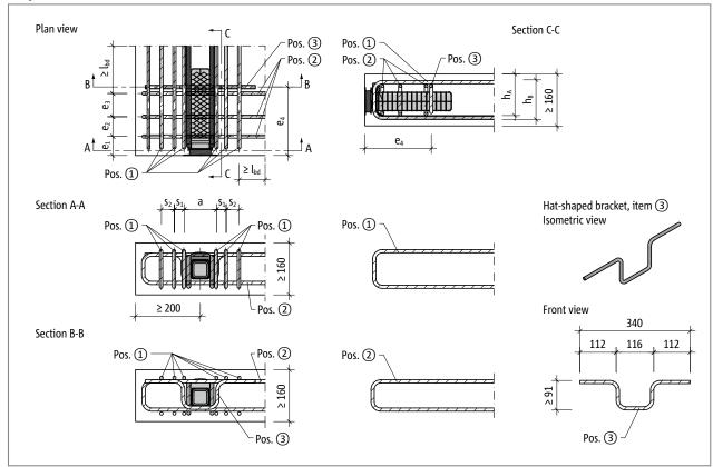
Fig. 136: Schöck Tronsole® Type P: On-site reinforcement
