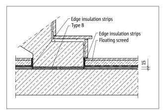
Fig. 16: Schöck Tronsole® Type B: Fire-protection version
