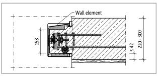
Fig. 150: Schöck Tronsole® type Z: Wall element as stay-in-place formwork; underside of the landing lower than the connection frame of the wall element
