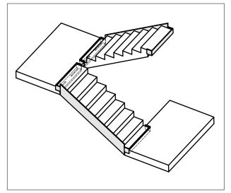
Fig. 13: Representation according to ISO 12354-2 of a flight of stairs separated from the landing and the floor
