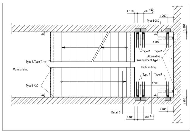
Fig. 128: Schöck Tronsole® Type P: Element arrangement in plan view using Tronsole® Type L
