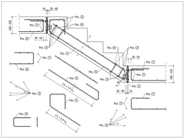
Fig. 48: Schöck Tronsole® type T: On-site reinforcement
