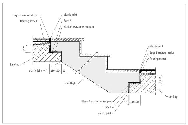
Fig. 65: Schöck Tronsole® type F: Installation cross section
