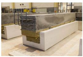
The insulation panels in the concrete sandwich facade are up to 35 centimeters thick. Photo: Schöck Bauteile GmbH
