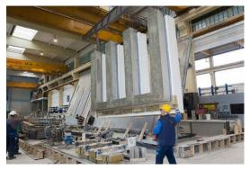
Schöck Isolink was able to guarantee the stable reinforcement of the cantilevered double-shell precast concrete components. Photo: Schöck Bauteile GmbH
