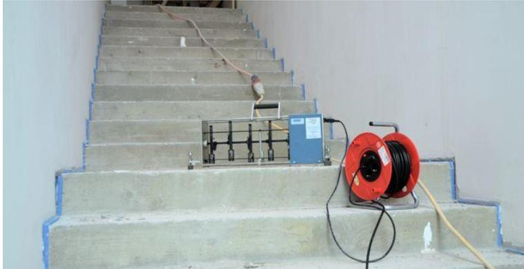
*Noise tests on site confirm the sound proofing achieved class 'A' and therefore the 'excellent comfort' classification. Schöck Bauteile GmbH*
