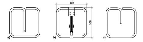
FIGURE 6—STAINLESS STEEL SPECIAL STIRRUP (DIMENSIONS IN MM)
