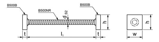
FIGURE 8—STEEL COMPRESSION BEARING (SCB)
