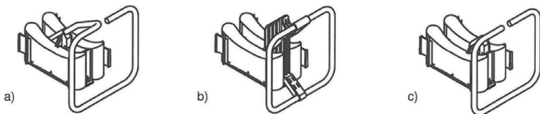
Fig 31 Concrete compression bearing with special stirrup
