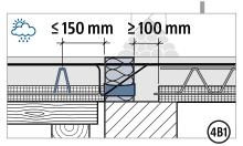
Be sure to fill the compression joint with in-situ concrete! Joint width ≥ 100 mm.
