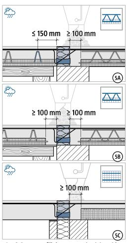
**5A–5C:** Be sure to fill the compression joint with in-situ concrete! Joint width ≥ 100 mm.
