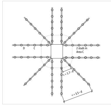
1: 12 rails are required due to the geometrical spacing rules
