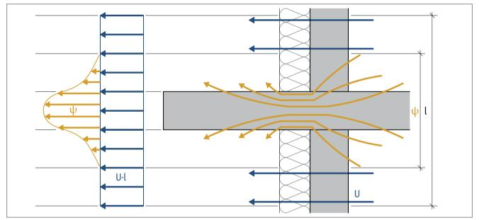
Figure 1: Pattern of heat flow through a building enclosure with materials that allow lateral heat flow to a thermal bridge
