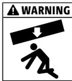
**WARNING** Hazard due to falling structural components with missing support! The balcony must always be supported statically designed. Remove temporary support only after installation of final support.
